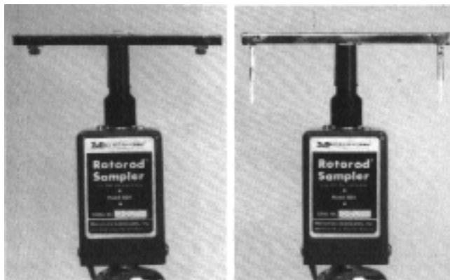
Fig. 3. Rotorod® intermittent sampler. The two sampling arms are folded onto a support bar; when the device starts rotating the sampling arms open vertically downwards and expose the impaction rods.
