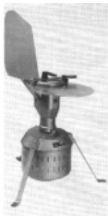
Fig. 5. The Burkard Seven-Day Volumetric Spore-Trap®. It is based upon the same principle as the Hirst device, but allows uninterrupted sampling throughout seven days.
